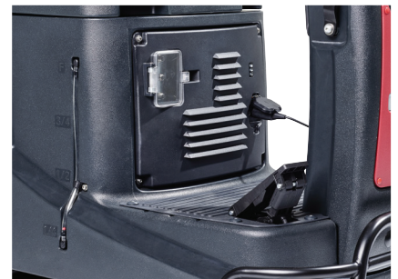
USB-port for fast charging of tablets and cell phones
