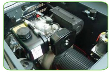
Available in petrol or diesel powered motorisations, including variable hydraulic traction power drive system.
