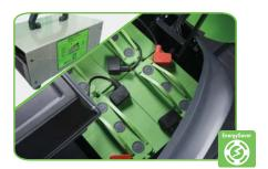
Batteries **Power Battery** with Gel technology which don't require maintenance. Very low levels of auto-discharge and made from almost completely recyclable materials.
